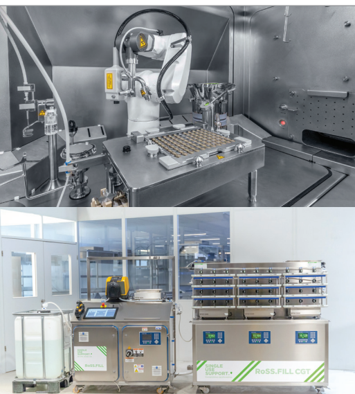
Figure 6. Crystal L1 robotic vial fill line (A) and Single Use Support ROSS.FILL CGT bag filler (B) (5, 6).
