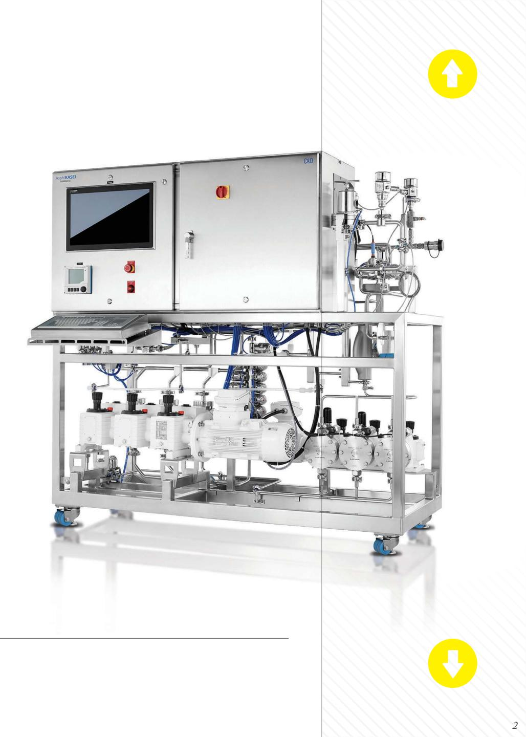
occurs in synthesis columns, while the synthesizer precisely delivers the amidites and all required reagents. The sizing and pairing of the synthesizer with the columns are key for effective coupling and yield.
