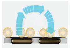
Figure 2: The electrodes detect small changes in the impedance of current flow caused by the cells' presence, attachment, and behavior
