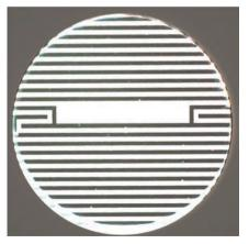
Figure 1: Interdigitated electrodes embedded in the cell culture substrate at the bottom of each well in a microtiter plate
