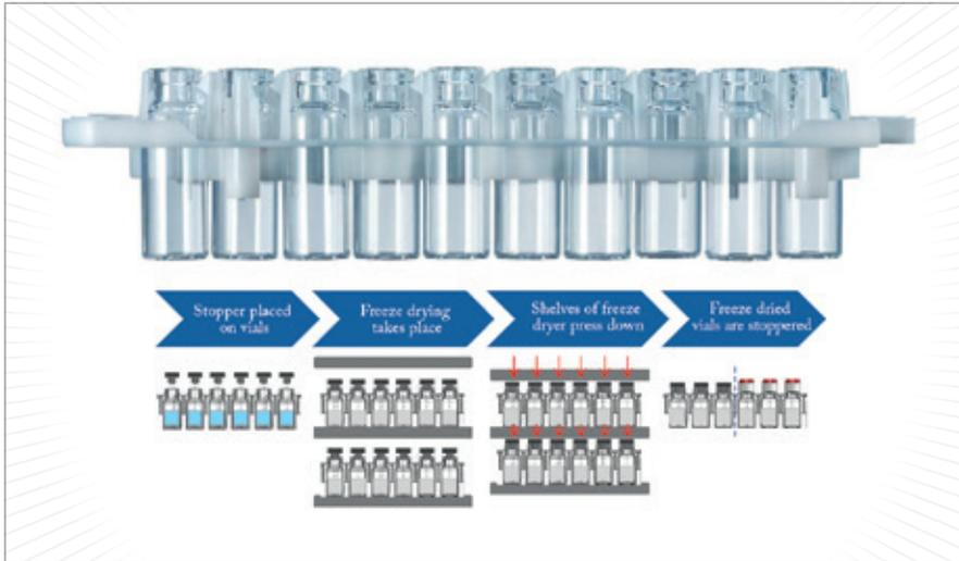
Figure 1. Freeze drying process.
